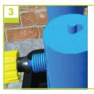
Remove collar Push 9mm pipe through collar and attach to AQUAvalve nozzle Rescrew collar - DON'T overturn... when you feel it grip **STOP**
